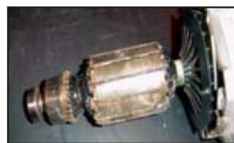
Armature burnt out (overloaded)
