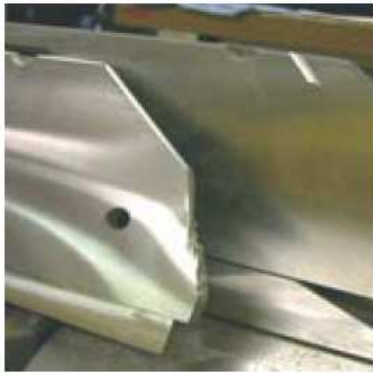
Abused fence - blade impact
