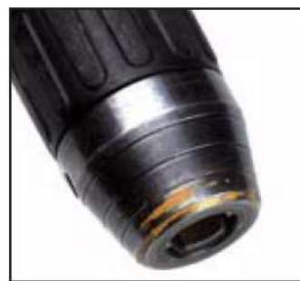
Wear caused by operating the drill with the chuck running against masonry or other hard surfaces
